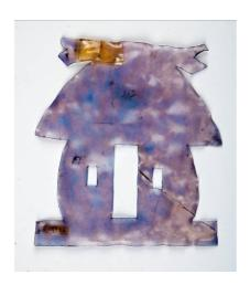
5.2.6 Stencils made from cellulose (film material)
